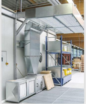
The grinding extractor is designed for extracting wood dust from manual grinding. Suction works over the entire working surface.
